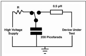
Figure 2: Typical Machine Model circuit diagram
