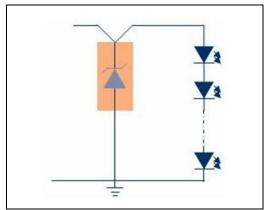
Figure 5: Adopting a reversed Zener diode in parallel with LED string
