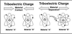
Figure 1: Principle of Triboelectric charge
