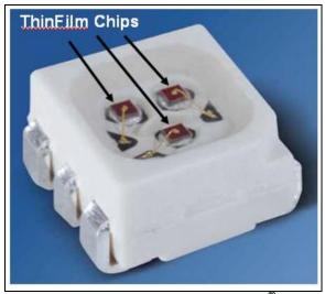
Figure 4: 6-lead Multi TOPLED<sup>®</sup> with Thinfilm Chips and no ESD protection diode, due to space restrictions
