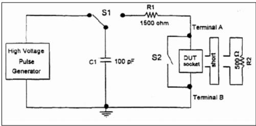
Figure 1: Typical equivalent HBM ESD circuit
