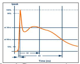
Figure 6: The most commonly used waveform of ESD discharge defined by IEC61000-4-2
